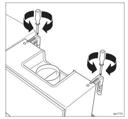
Using the screws of the adjustable brackets, you can align the unit with the height of the adjoining cabinets. Turn them
